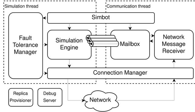
**Fig. 3.** Simbot Architecture for Fault Tolerant Simulation
